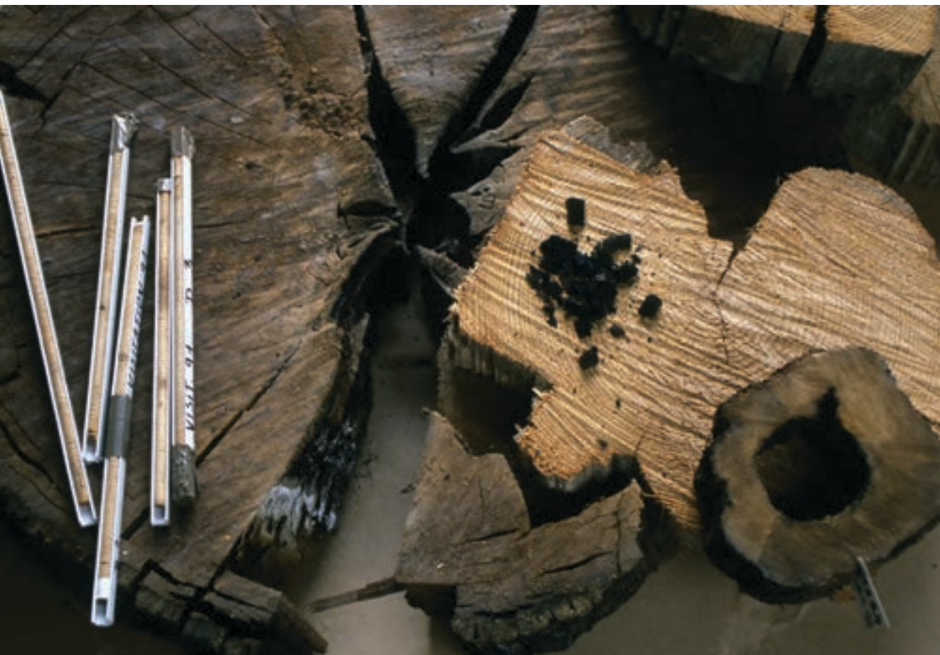
Equipment for sampling ancient wood for dendrochronology © Hervé Paitier, Inrap
