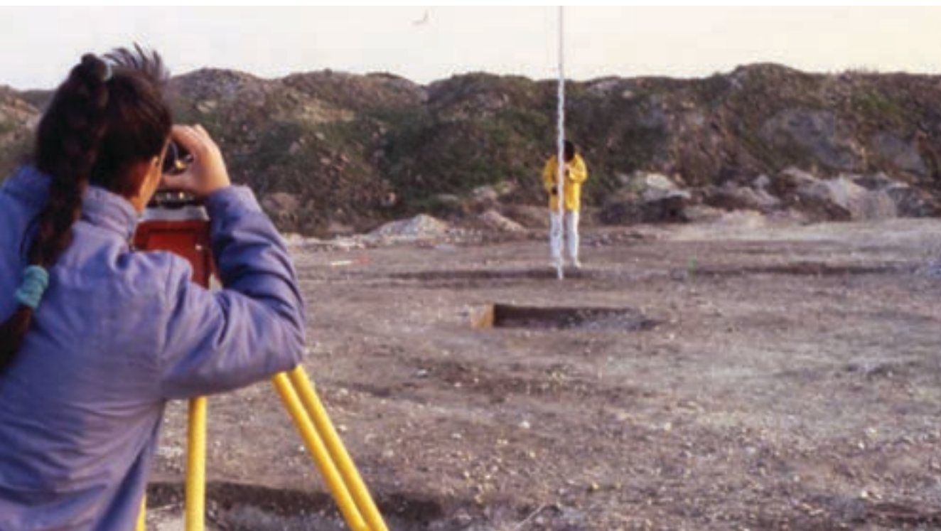
Recording the levels on the site of Fresnes-lès-Montauban, using a theodolite © Inrap
