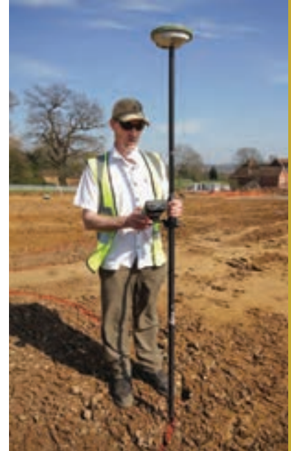
Surveying with GPS (Kent, England) © Canterbury Archaeological Trust
